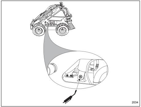
Figure 4-10 Loader Arm Lift Cylinder Base Lubrication Point
